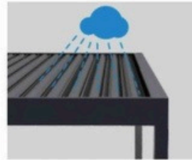
Rubber strip built into blades To reach 100% waterproof
