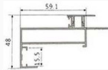
DOUBLE PACK ( PEVERSE SIDE ) (WAU THICKNESS: 1.4MM)
