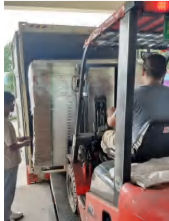
Load the door into the container with a forklift
