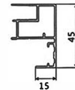
DOOR LINE (WALL THICKNESS: 1.4MM)
