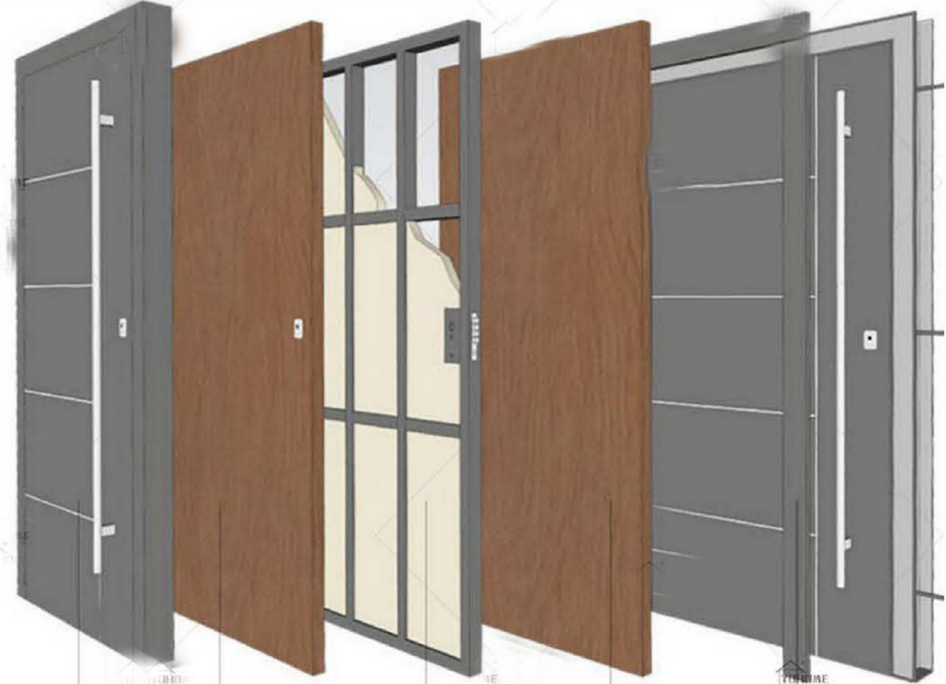
STAINLESS STEEL BOARD 10mm PLYWOOD HEAT INSULATION FOAM 10mm PLYWOOD DOOR CASE
